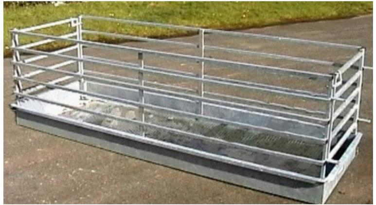
This footbath was designed for the zinc sulphate solutions similar to 'Golden Hoof' foot rot treatment for sheep. The fully galvanised unit incorporates an eight inch deep galvanised steel footbath with 2089 expanded metal sheep mesh for a non slip surface. The system is easily dismantled into three sections to take up minimal space when transporting or storing.
